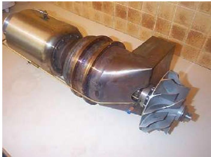
**Figure 1: Microjet Engineering Turboshaft Engine**
