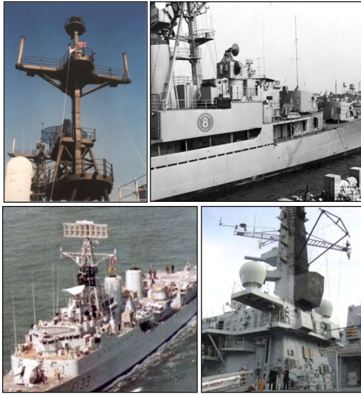
Figure 1: Illustrations of Mast Types – Pole (top left), Tripod (top right), Lattice (bottom left), Plated (bottom right)
