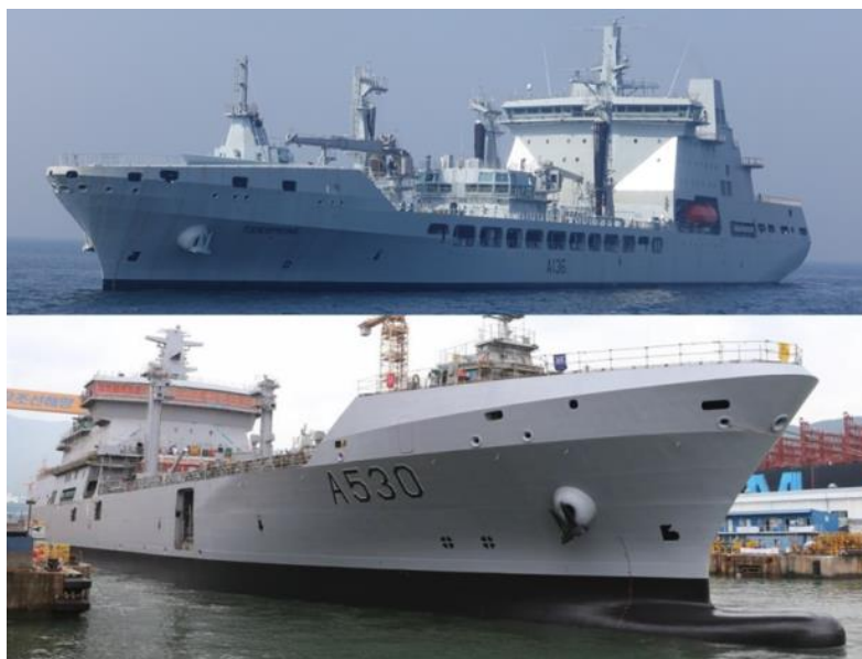
Figure 2: (top) BMT Aegir® design for the UK Tide Class designed to Lloyd's Register naval rules. (below) BMT Aegir® design for the Royal Norwegian Navy designed to DNV naval rules.
