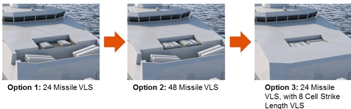
Figure 4: Example of VLS options within a Light Frigate design, which could be adopted over a class of ships to provide greater capability once the initial risks are resolved or mitigated.
