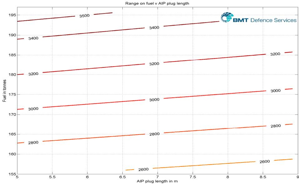
**Figure 3: Range on Fuel v AIP plug length**
