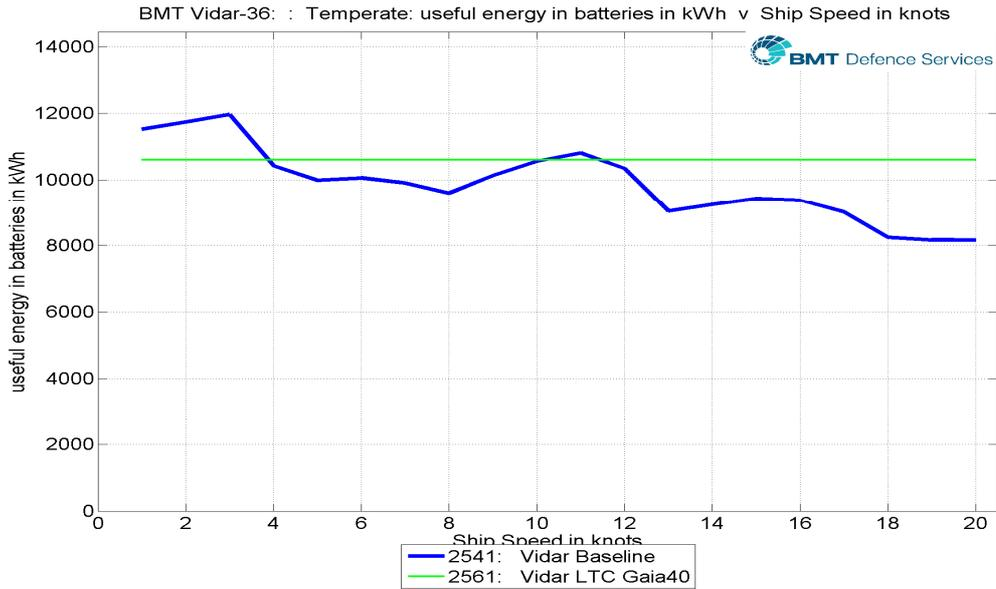
**Figure 4: Useful Energy Stored in Ship’s Battery**
